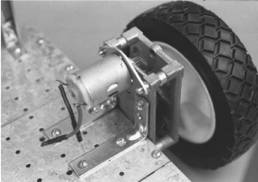
FIGURE 21.4 One of the drive motors, with wheel, attached to the base of the Roverbot.
