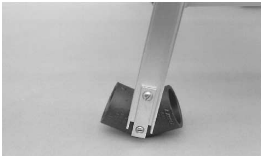
FIGURE 22.14 PVC plumbing fittings used as feet. The feet use a flat mending iron. Add pads or rubber to the bottom of the feet as desired.
