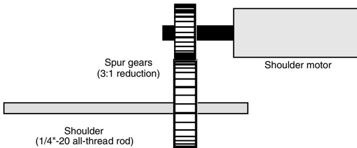
**FIGURE 25.1** The gear transfer system used to actuate the shoulder of the revolute arm. You can also use a motor with a built-in reduction gear if the output of the motor is not slow enough for the arm.
