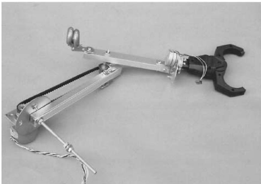
**FIGURE 25.7** The completed arm, with gripper (hand) attached.
