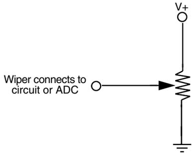
**FIGURE 25.11** The basic electrical hookup for providing a varying voltage from a potentiometer.
