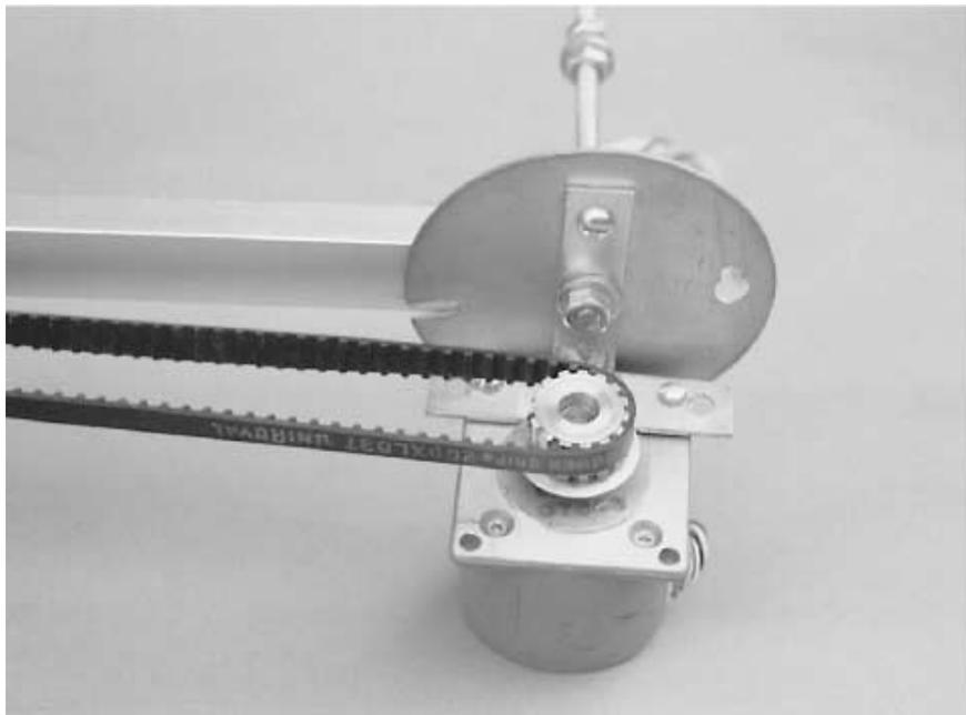
**FIGURE 25.6** The motor mounted on the shoulder.
