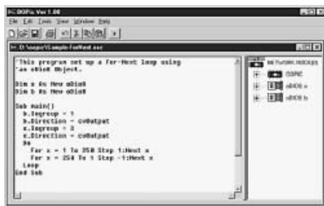
FIGURE 33.4 Programs are written for the OOPic using a Windows-based software development platform. You open, save, debug, and compile your OOPic programs using pull-down menu commands.
